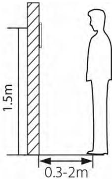
The distance between the device and a user whose height is within 1.55m-1.85m is recommended to be 0.3 to 2m. Users may slightly move forwards and backwards to improve the quality of facial images captured.
